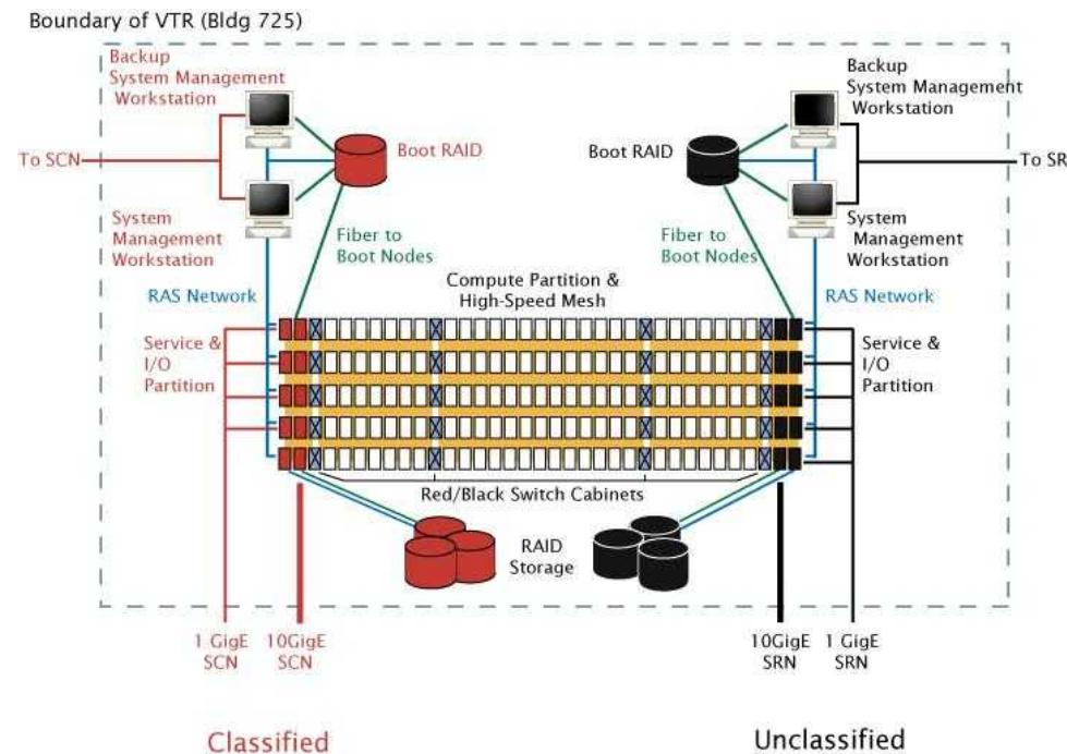
5th row added bringing node count to 3360 on the unclassified side and 3360 on the classified side. The middle section contains 6240 nodes. Total number of compute nodes at 12960. Each compute node upgraded to dual core technology, bringing total processor count to **25920**.
