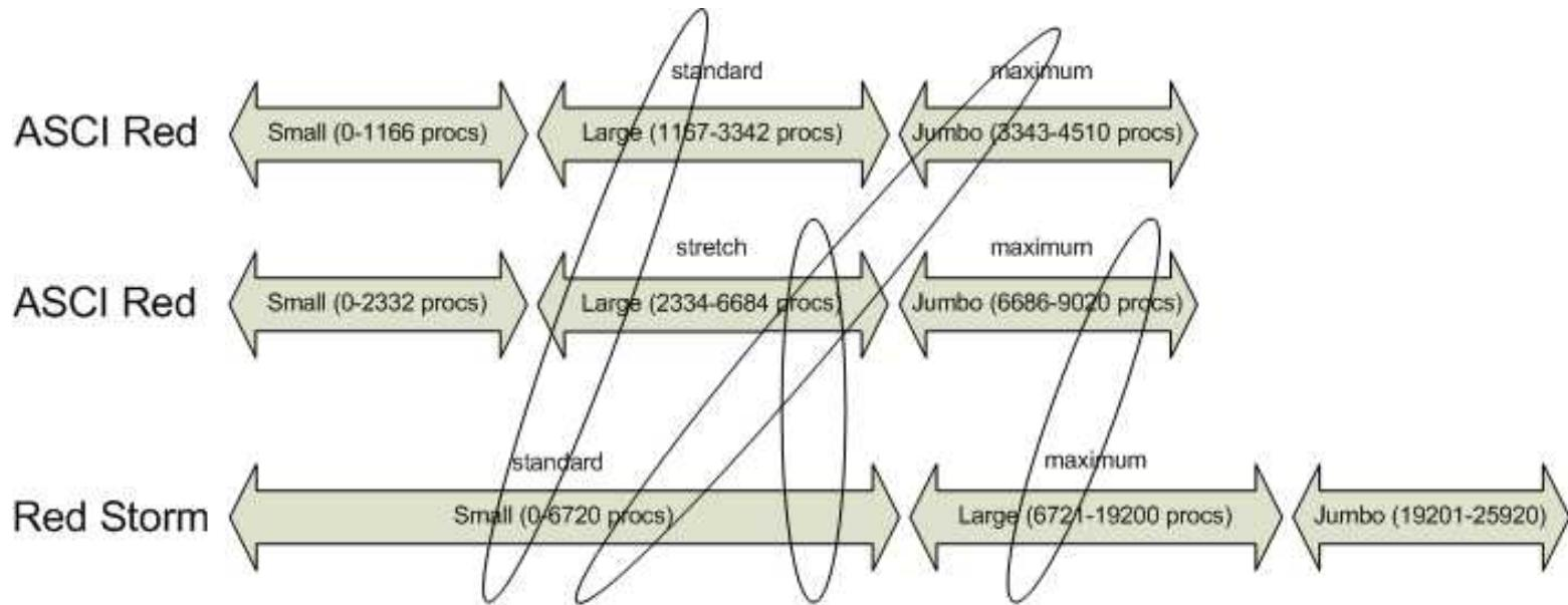
ASCI Red: 4510 compute nodes (9020 processors). Proc 0 mode uses one processor per node and the full 256 MB of memory. Proc 3 mode uses two processors per node but only 128 MB of memory is available to each process.
