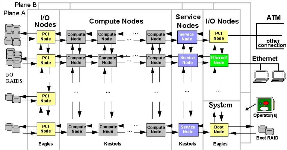
1168 nodes on the unclassified side and 1166 nodes on the classified side. The middle section contains 2176 nodes. Total number of compute nodes at 4510. Each compute node contained 2 processors, bringing total processor count to **9020**.
