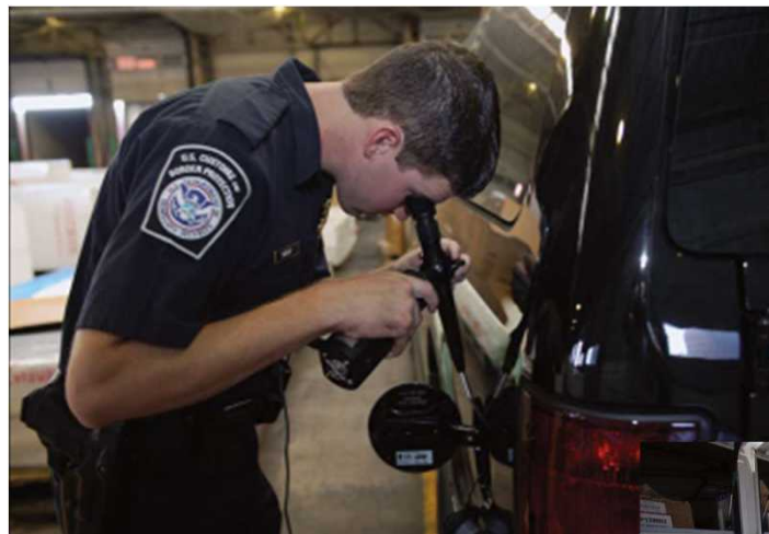
Fiber-optic tool to look inside enclosed spaces
