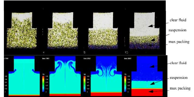
**Figure 1. Particle Settling in a Cylinder with a Contraction for 0.192 volume fraction of 0.0397cm radius PMMA particles in a glycerol and water suspending fluid. Particles are slightly heavier than fluid : a) NMR imaging at  $t=105.s, 175s, 315s, 560s$  b) Finite Element Simulations at  $t=110s, 190s, 310s, \text{ and } 590s$**
