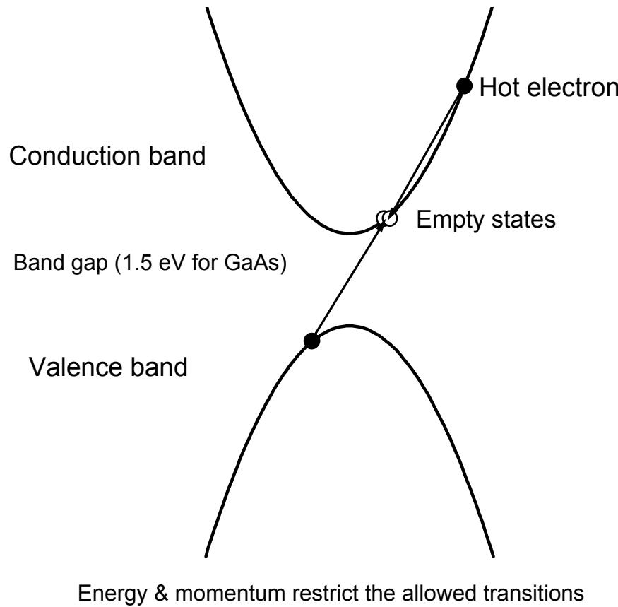
An electron heated by the electric field generates another electron and a hole
