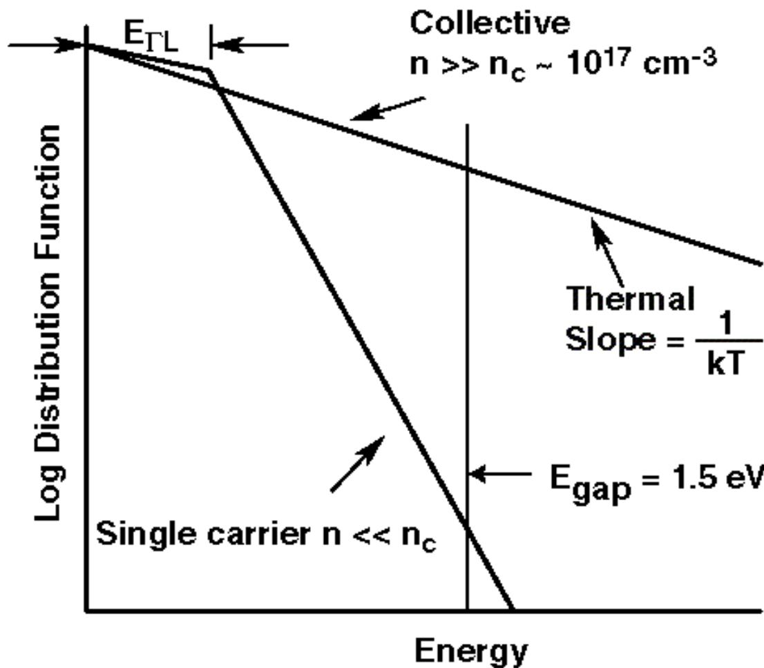
The tail of the distribution function generates electrons and holes by impact ionization
