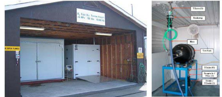
Powertech's 70 MPa fast fill test facility equipped with hydrogen-safe environmental chambers.
