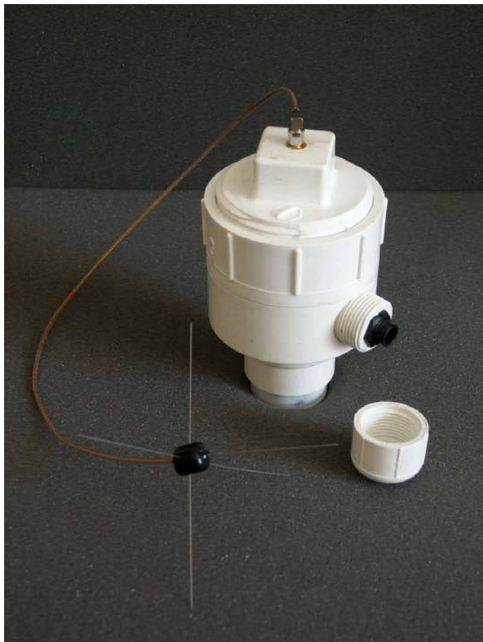
SCSN with ground-mounted antenna and dust cap removed from 18-pin connector
