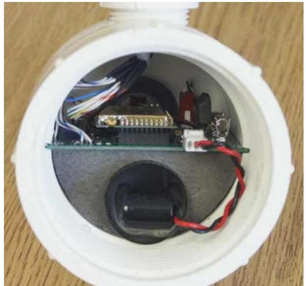
Interior view showing D-sized battery and printed circuit board with radio and microprocessor. The geophone and inertial switch are not visible.
