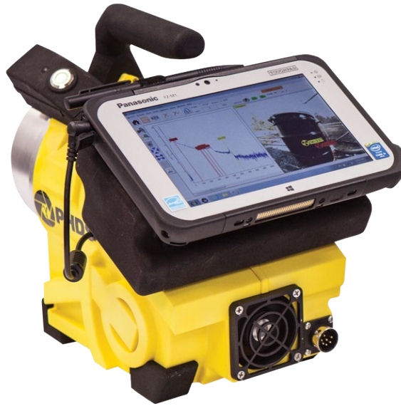
Figure 2. GeGI, PHDS' germanium gamma ray imaging system
