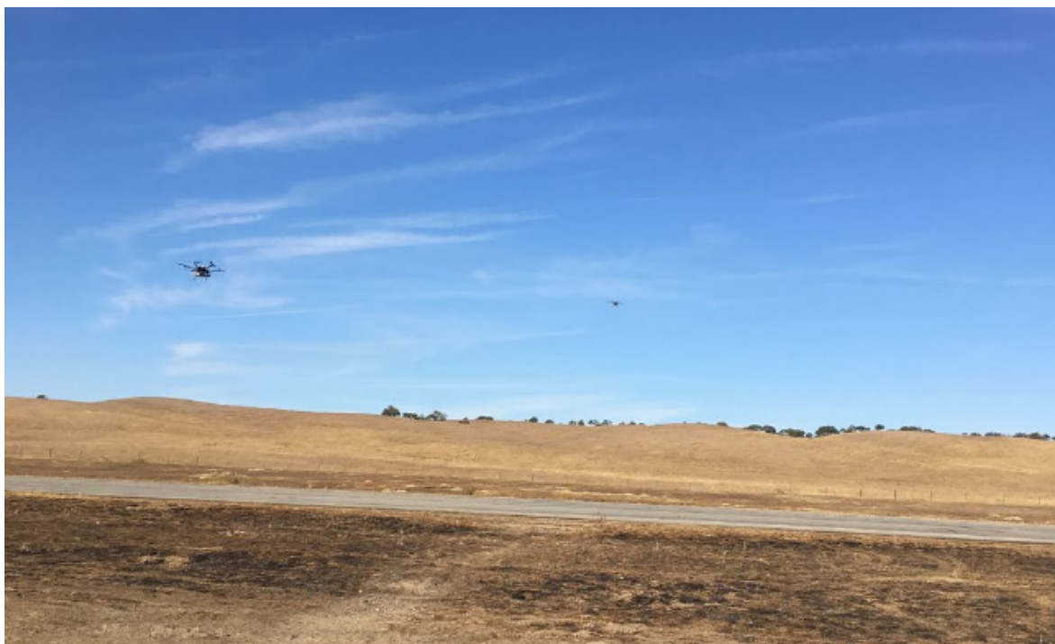
Figure 29. After the incident that disabled the Albatross, a second Harris H6, seen in the distance, was used as the communications relay. The hexacopter carrying the 3×6 NaI detector pod is in the left foreground.
