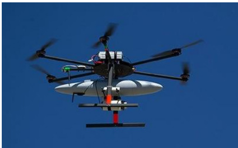
Figure 9. Va Tech hexacopter carrying the Apollo gamma imager pod and the 2x2 NaI detector mounted beneath the pod
