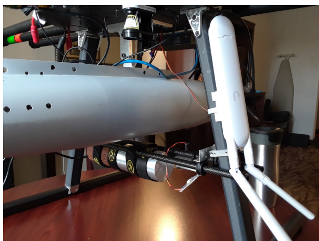
Figure 11. Close-up of the Apollo pod and the 2x2 NaI detector mounted beneath the hexacopter with the LIDAR at the top, and the 2.4 GHz Ubiquiti radio mounted on the landing strut in the right foreground.
