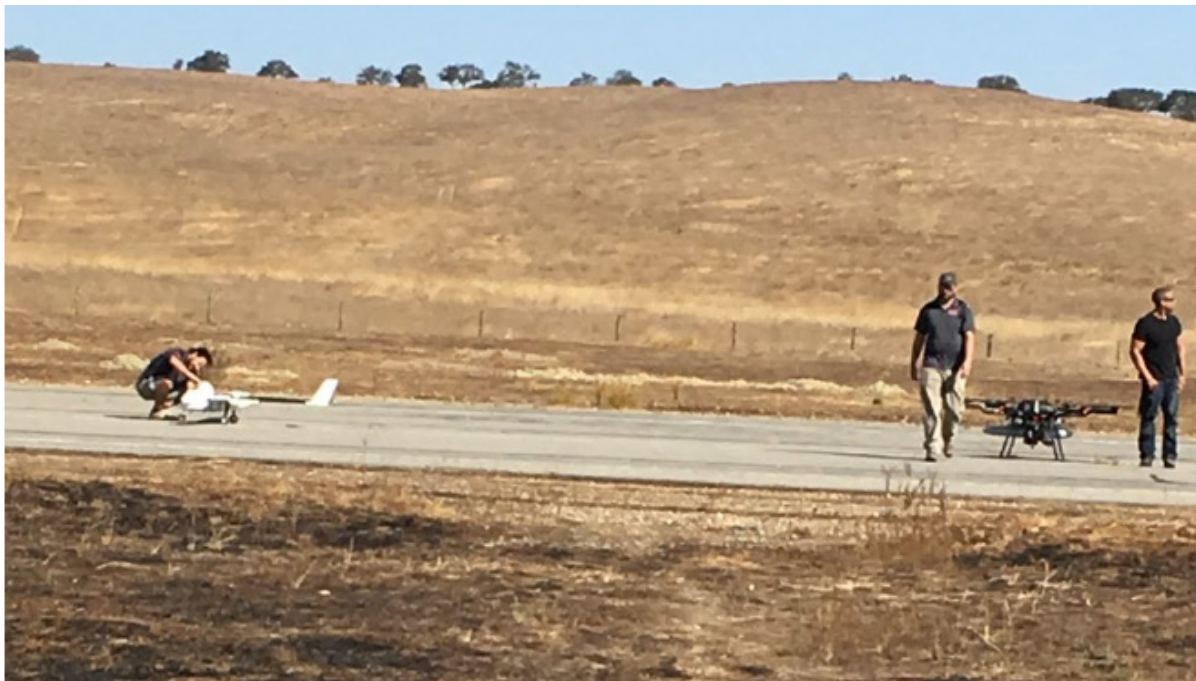
Figure 27. At the left is the Albatross fixed-wing sUAS, which was intended to be a radio communications relay. On the right is the Harris H6 hexacopter that flew the survey pattern.
