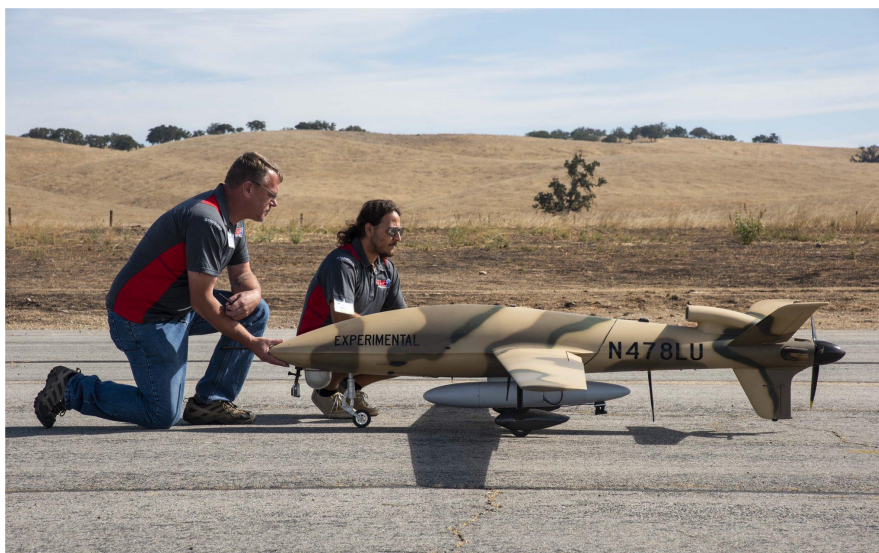
Figure 21. The USI Sandstorm on the McMillan runway with the detector pod attached to the belly of the fuselage. Todd Bagley (left) and Hovig Yaralian (right) of USI are completing final checks before flight.
