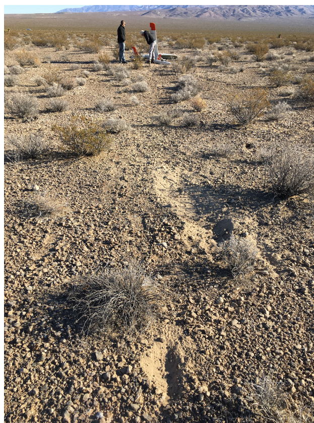
Figure 3. The Sandstorm was banking into a turn when it lost power. Marks in the terrain show the wing and fuselage impact.
