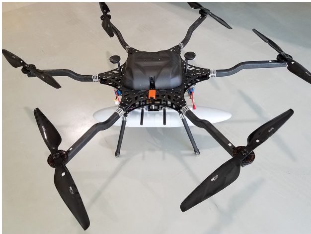
Figure 26. The Harris H6 hexacopter has a gasoline-powered generator to maintain battery charge for two hours of flight. It is shown here carrying the STL 3×6 NaI radiation detection pod.
