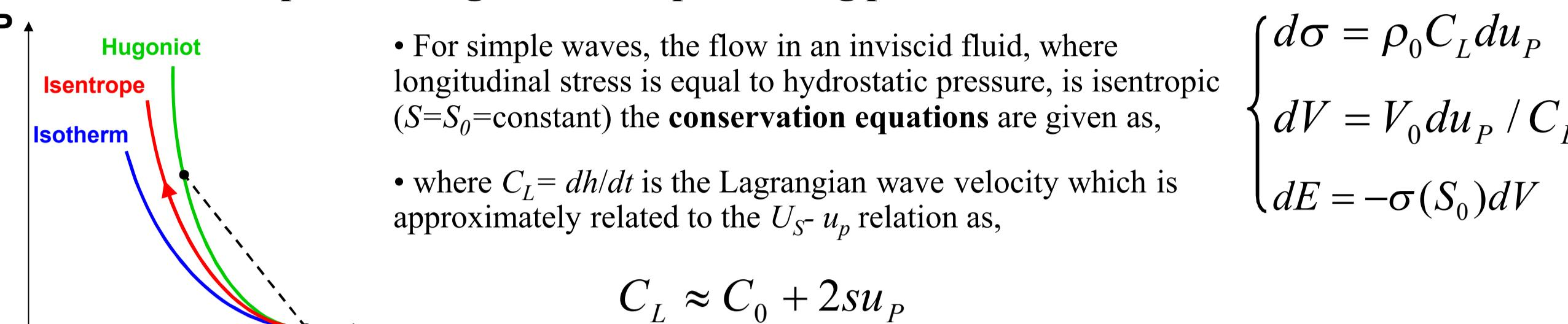
Stress-strain loading paths can be determined continuously to peak pressure for most materials.
