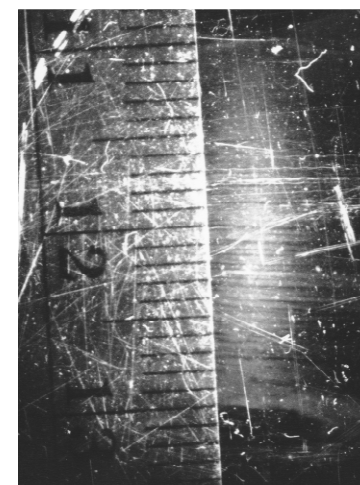
0.25mm - 1.0mm Striations Observed on Insulator Positioned 1mm from Wire
