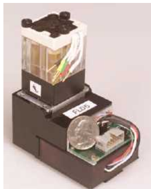
Liquid Phase \mu ChemLab TM for Fluid Analysis
