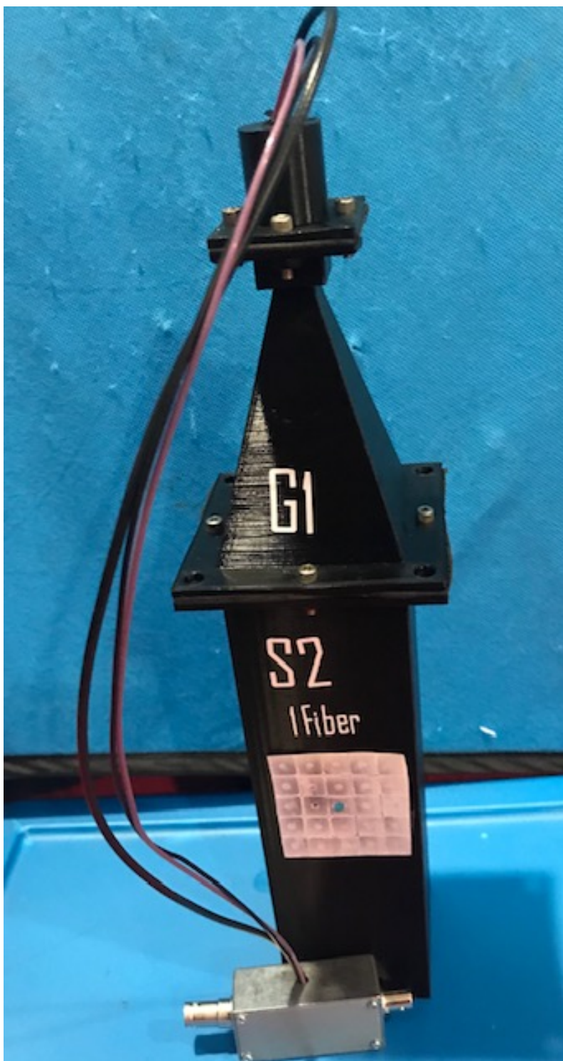
Figure 8: Final assembly of one-pixel detector unit.
