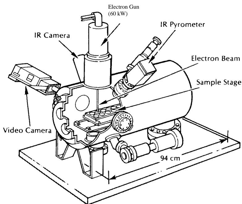
FIGURE 1. EB-60 SCHEMATIC
