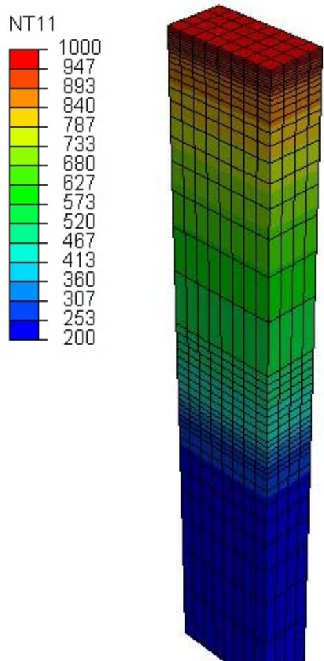
**1-D analysis with k-eff for mesh and temperature dependent properties**
