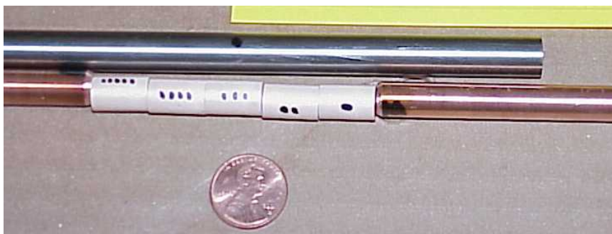
Cerium Oxide ceramic surrogate pellets, Zircaloy cladding tube / test rod
