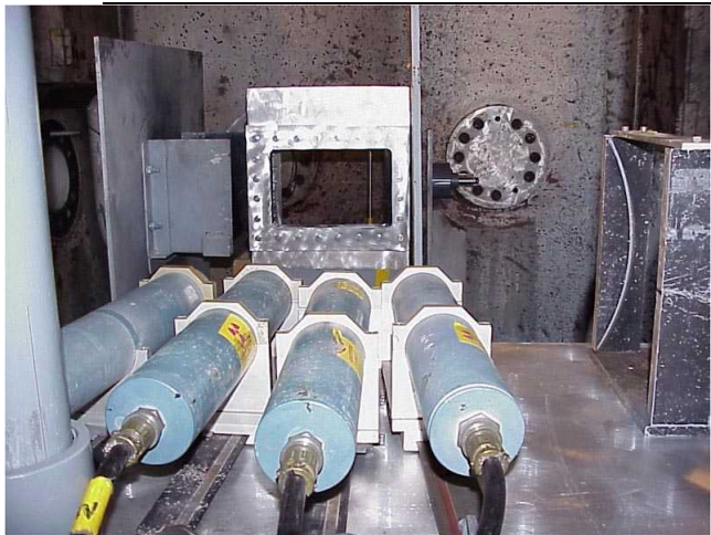
ECF test pad ↑ 4 flash X-ray tubes
