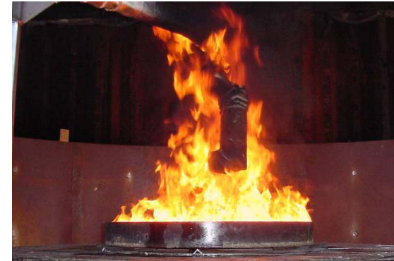
Diode laser diagnostic probe taking measurements in 1-m diameter JP-8 fire (FLAME facility, SNL/NM, Sept. 2000)
