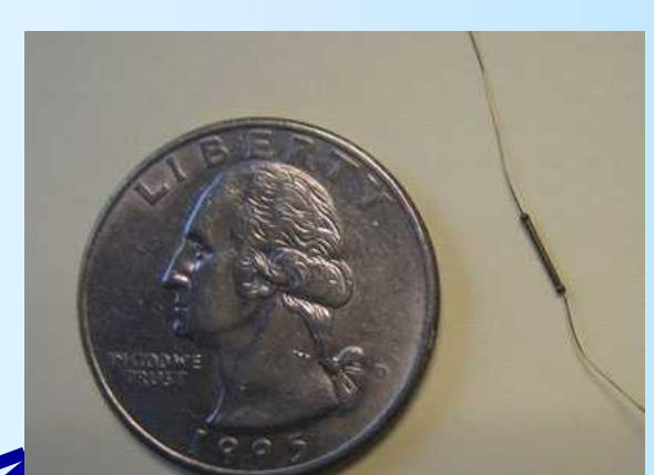
**Programmable Integrated Circuit (PIC)** formed the bottom plain of the system and was fabricated out of a commercial MicroChip 16C622 PIC. The chip was programmed prior to de-packaging and thinning to nominally 100 microns.
