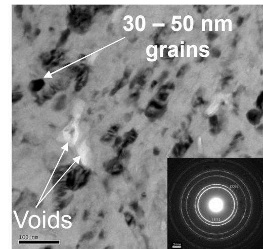
Cold Sprayed LN<sub>2</sub> Ball Milled Al 6061 Powder has 30-50nm grains and small regions of porosity
