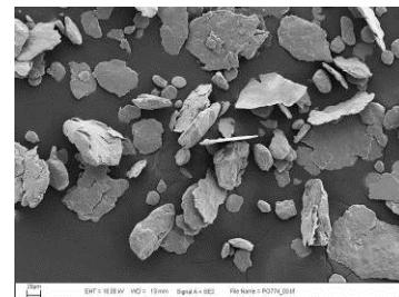
LN<sub>2</sub> Ball Milled, Nanostructured Powder
