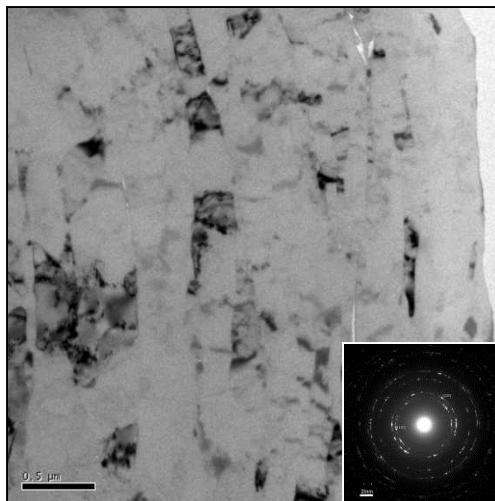
LN<sub>2</sub> Ball Milled Al 6061 Powder Has 250-300nm grains, lath-like structure w/ intra-grain porosity and no texture
