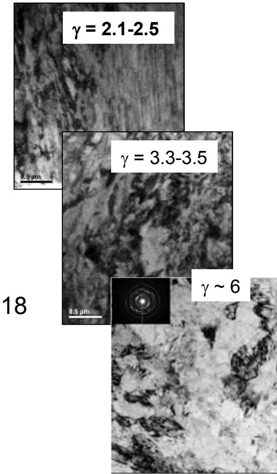
Large Strain Extrusion
