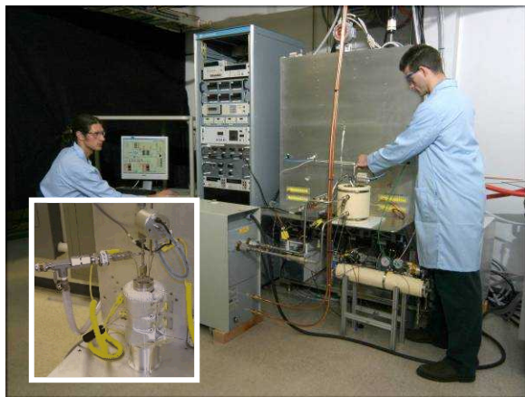
Figure 5 - Large Sieverts-type hydride station with prototype solid-state hydrogen storage systems
