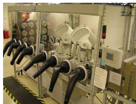
Figure 4 - Inert glove box utilized for the production and handling of reactive hydrogen storage materials
