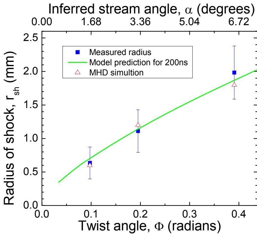
Experimental data indicates hollow conical shock
