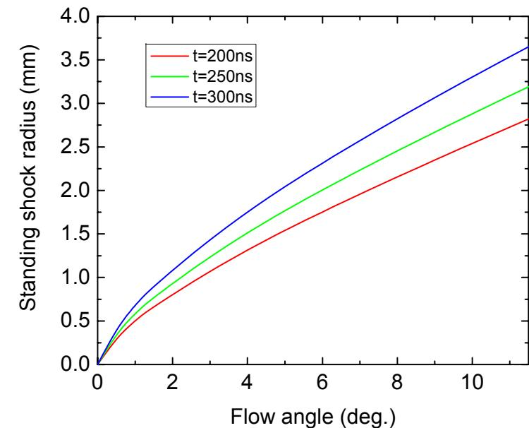
Expect the diameter of the conical shock to be approximately proportional to the flow angle (and hence also to the angle of twist between the two electrodes)
