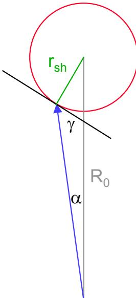
Standing shock radius is determined by the balance between the centrifugal force of the rotating shock and the kinetic pressure of the converging plasma acting on the surface of the shock:
