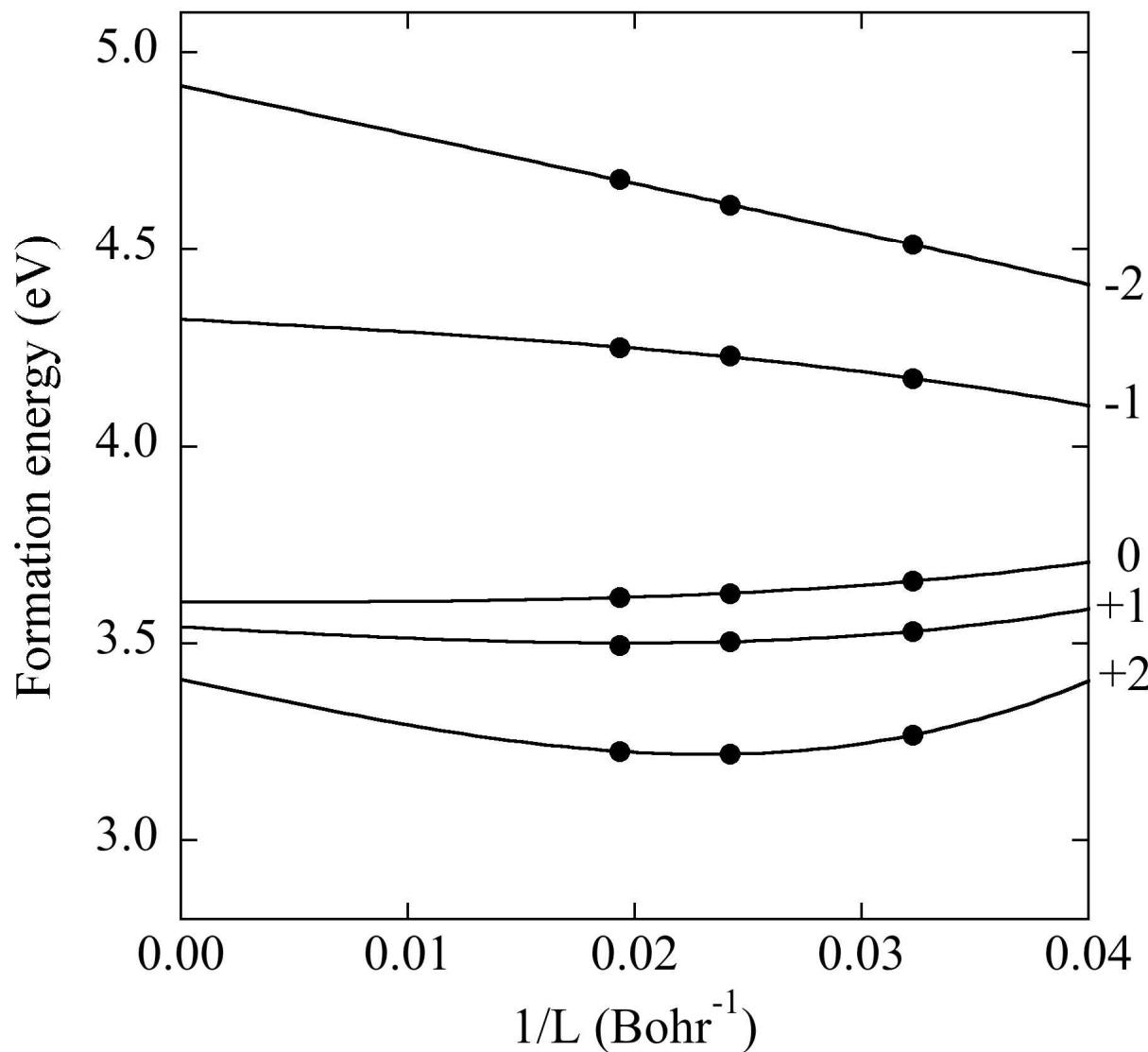
Fits to the supercell formation energies of Si vacancy saddle points obtained in simple cubic supercells using the UBC method and the PBE
