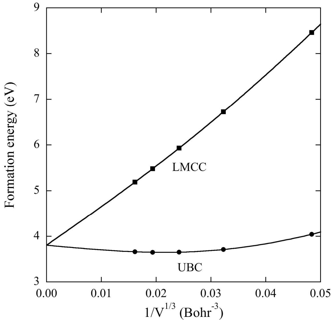
Fits to the supercell formation energies of the unrelaxed +2 Si self-interstitial obtained in simple cubic supercells using the UBC and LMCC methods
