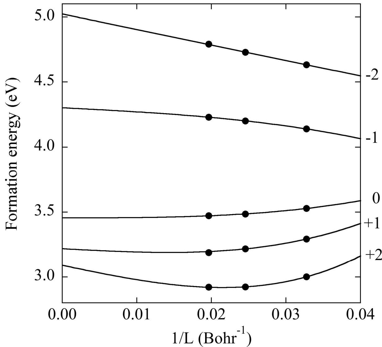
Fits to the supercell formation energies of relaxed Si vacancies obtained in simple cubic supercells using the UBC method and the PBE
