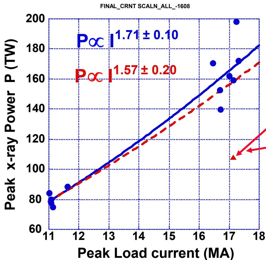
One shot Z\_1608 (load installed at midnight) gave very low power for no apparent reason. However it substantially affected the power scaling by more than  $1\sigma$ .
