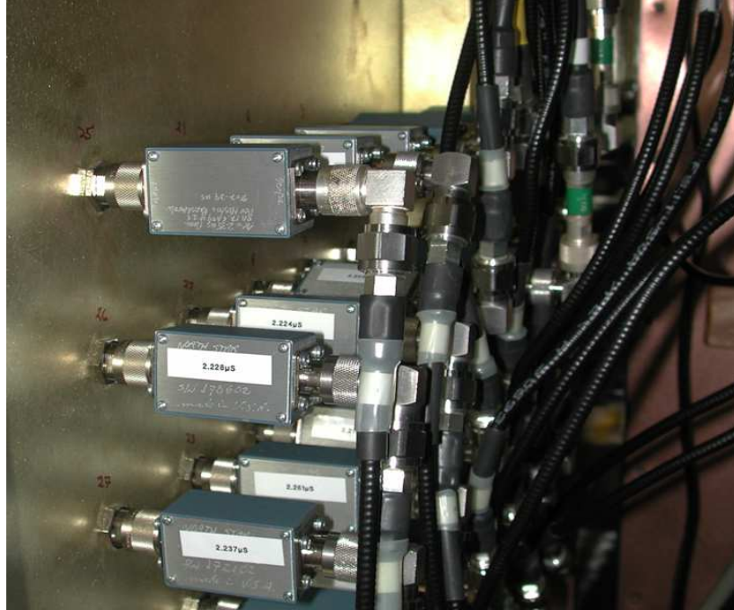
Figure 3.16: RC passive integrators. There is a single calibrated integrator for each of the 24 B-dot signals.
