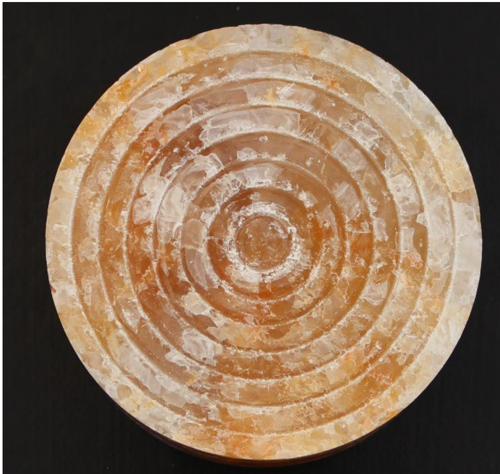
Figure 2-1. Grooves machined into a face of a 4-inch-diameter salt subcore.
