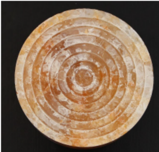
Figure 1. Grooves Were Machined Into One Face of Each 4-Inch-Diameter Salt Subcore.
