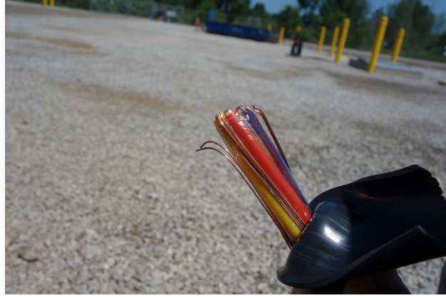
Figure 2.5.1. Sparse wire shielding found at some substations.
