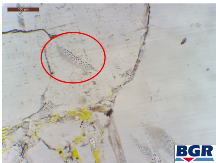
Fig. 4.53 Fluid inclusion planes (red circle) in compacted crushed salt. Scale bar is 100 \mu\text{m} .
