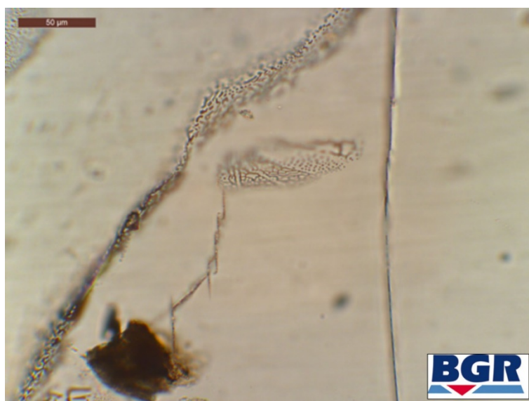
Fig. 4.55 Connected fluid inclusions in compacted crushed salt. Scale bar is 50 μm
