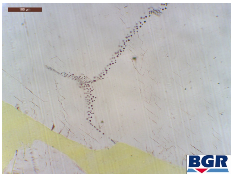
Fig. 4.5 Halite grain in uncompact crushed salt with en-échelon and fluid inclusion planes. Scale bar is 100 μm
