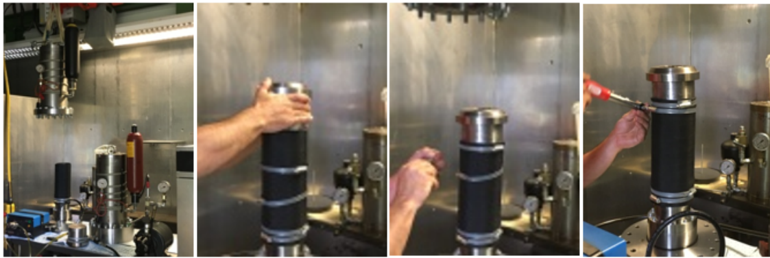
Fig. 4.17 Installation of crushed salt test pieces in autoclaves
