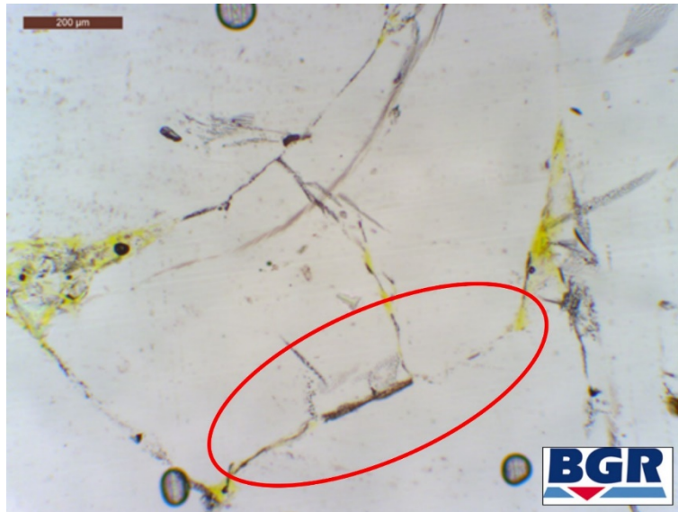
Fig. 4.56 Indicators for grain boundary diffusion (rounded grain edges with even grain contact, red circle) and compaction fringes in compacted crushed salt. Scale bar is 200 \mu\text{m}
