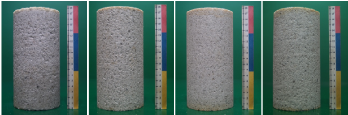
Fig. 4.22 Cylindrical test specimen with plane-parallel end faces and smooth lateral surface after machining on a lathe
