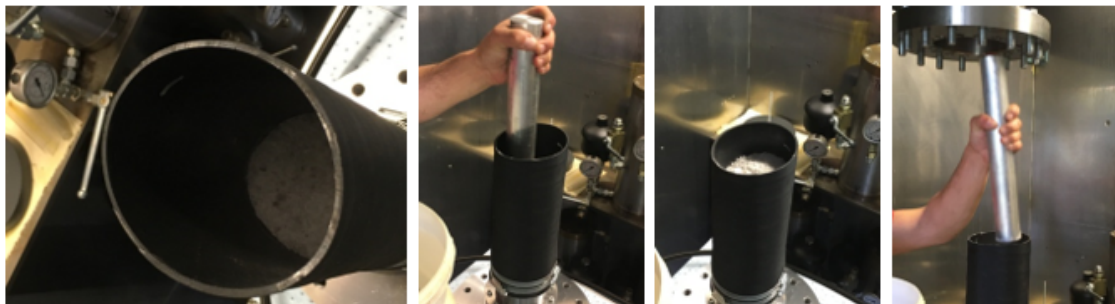
Fig. 4.16 Production of crushed salt test specimens for the pre-compaction by layer installation with moderate pre-compaction
