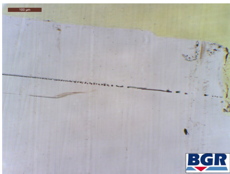
Fig. 4.6 Halite grain in uncompact crushed salt with two fluid inclusion lines, connected by a relay. Scale bar is 100 μm
