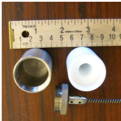
Fig. 3. Photograph of the tungsten AmLi source holder (left) and the ^{252}\text{Cf} HDPE source holder (right), beside the Teleflex cable-lid for transferring the sources into the AEFC in 2014.
