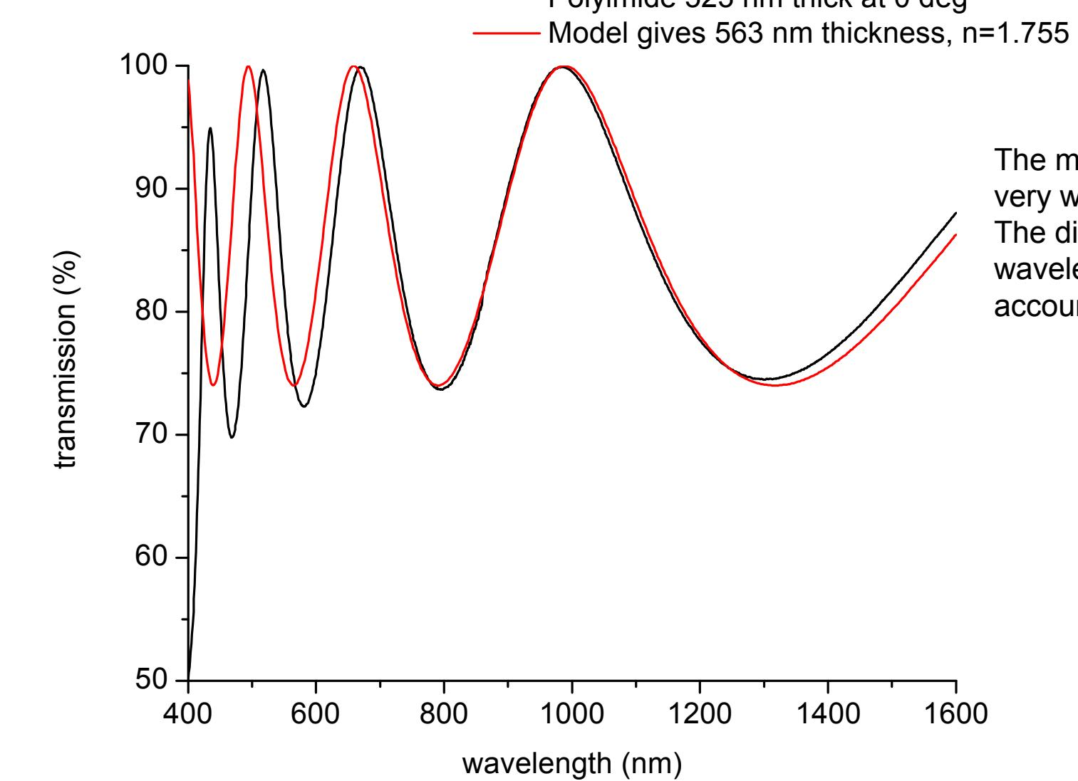
The model fits the data very well around 1054 nm. The discrepancy at lower wavelengths is due to unaccounted dispersion.
