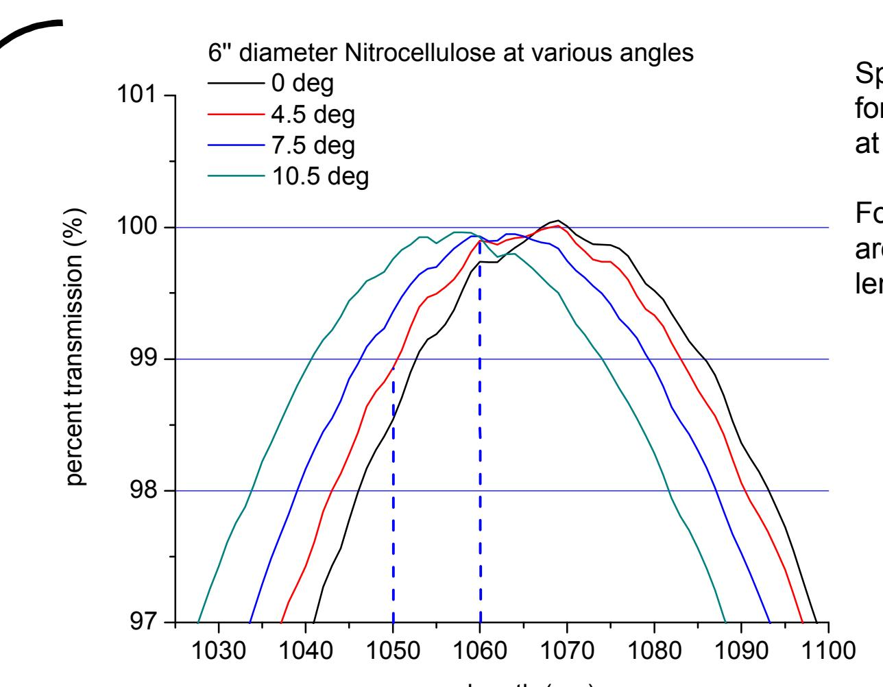
Spectral Photometer trace for a 6" Nitrocellulose pellicle at various angles of incidence.
