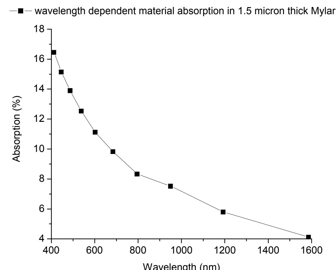
Material absorption is quite high. The lowest value of 4% is still above the highest absorption of 2.5% in nitrocellulose.
