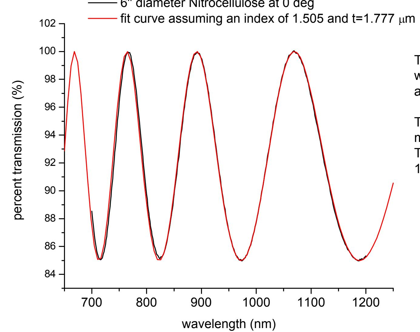
The theoretical prediction fits well with the data, using  $n=1.51$  and a thickness of 1.78 micron. The variation of the maxima and minima are due to material dispersion. The transmission is on the order of 100% over the range of 750-1200nm.
