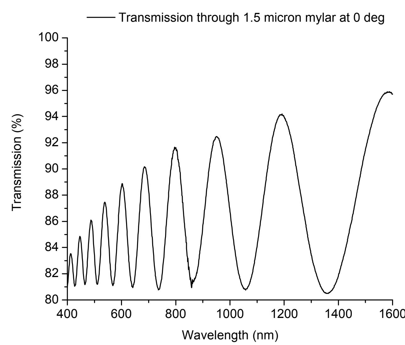
The spectral transmission curve shows an interference pattern typical for thin films. One can clearly see that Mylar exhibits an increased absorption towards shorter wavelength.
