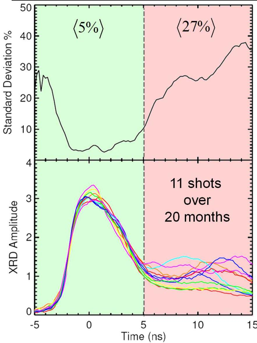
$$\frac{dV_{xrd}}{V_{xrd}} \approx \frac{\partial P_{DH}}{P_{DH}} \sim 5\%$$
