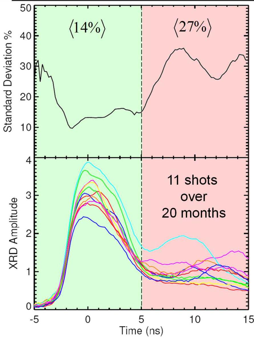
$$\frac{dV_{xrd}}{V_{xrd}} = \sqrt{\left(\frac{\partial P_{DH}}{P_{DH}}\right)^2 + \left(\frac{\partial \text{Inst.}}{\text{Inst.}}\right)^2} \sim 15\%$$
