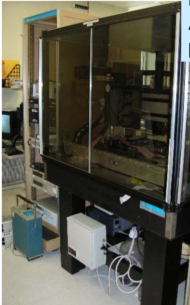
SHiMMeR 1 - Sandia High-volume Measurement of Micromachine Reliability
