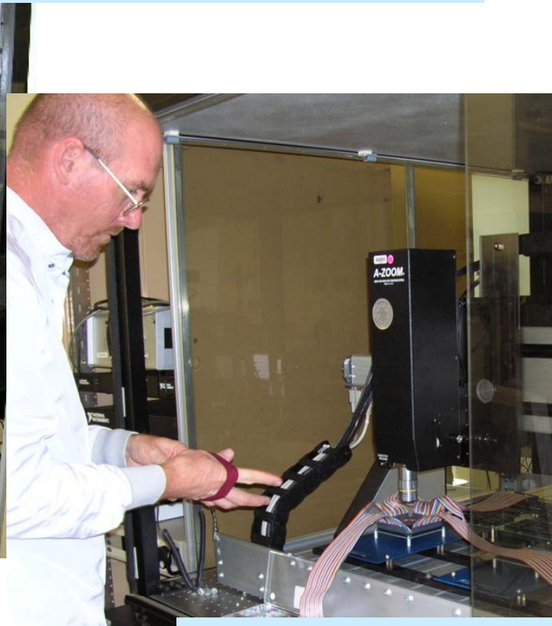
Gantry-Mounted Microscope, Automated positioning and control for inspection
