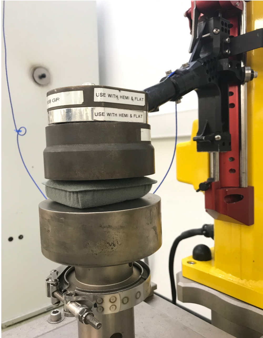
Figure D-6. Test configuration for compression of the Team Wendy helmet pad.
