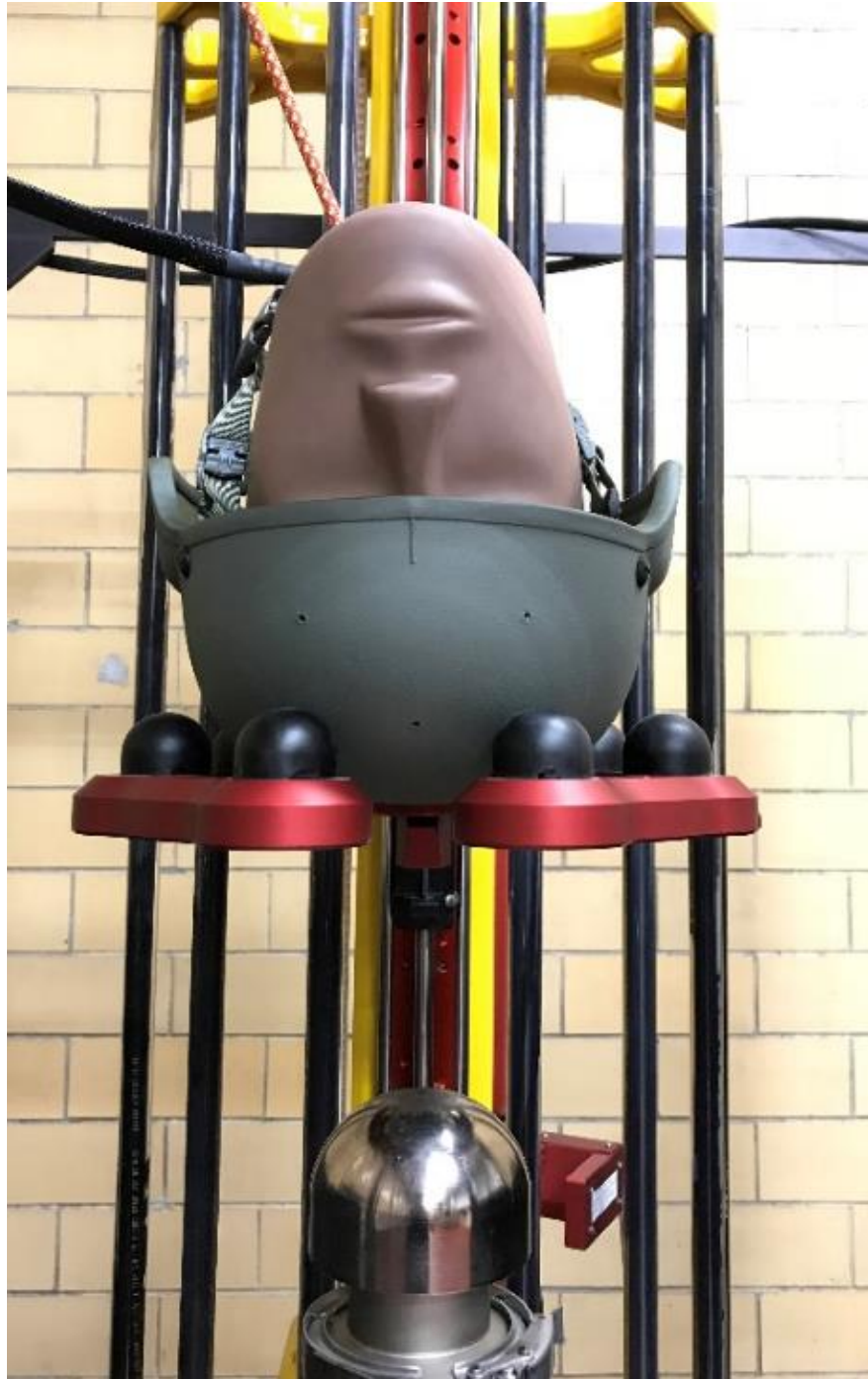
Figure 2-1. Mil-spec experimental setup, with hemispherical anvil.
