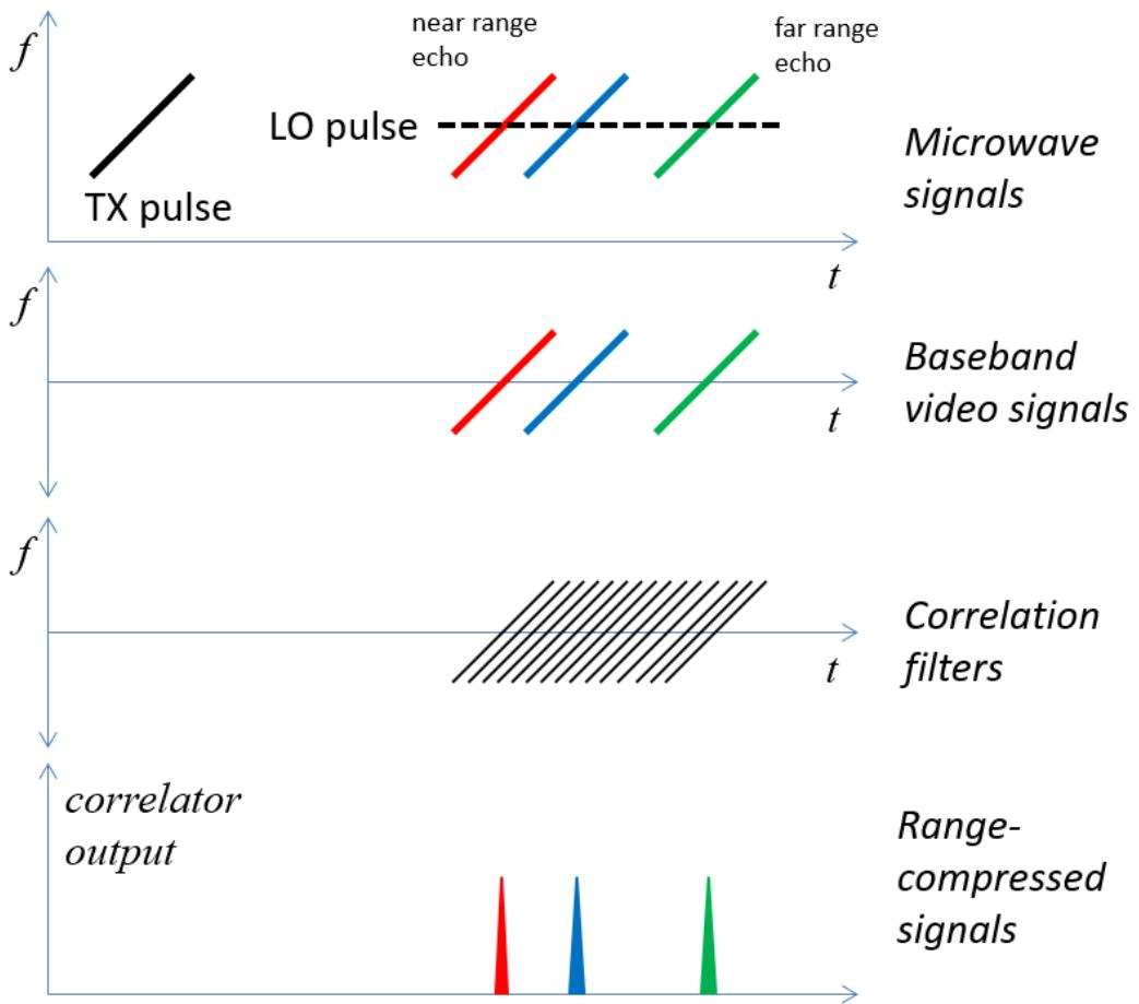
**Figure 1.** Pulse compression via correlation filters is indicated when the range swath is a large fraction (or larger) of the TX pulse width, or for coarser range resolutions. Note that the baseband video signal bandwidth is the same as the microwave signal bandwidth. This model applies to other waveforms, too.
