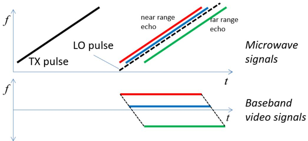
After de-ramping the echo energy with a LO pulse that is also a chirp, range is encoded in baseband video frequency. Consequently a DFT will separate frequencies, and hence ranges.
