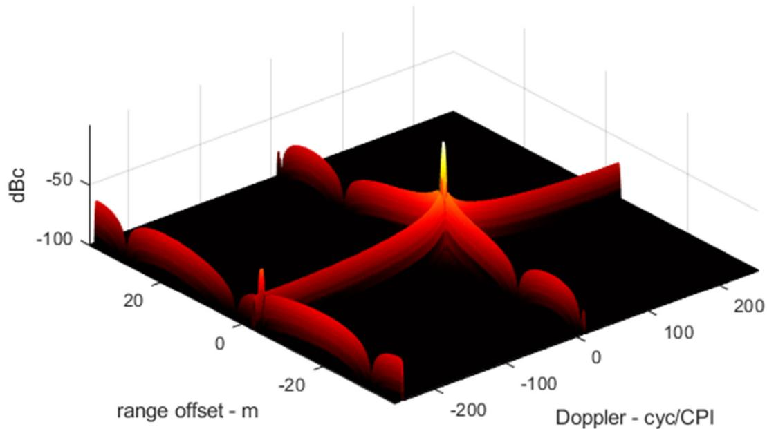
**Figure 4. Example IPR of CPI using alternating up-chirp and down-chirp, using stretch processing.**
