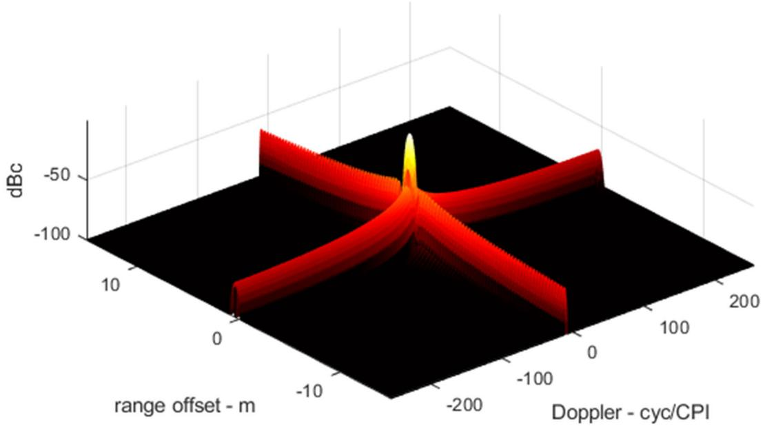
Figure 3. Example IPR of CPI using alternating up-chirp and down-chirp, using correlation processing.
