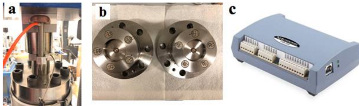
Figure 2-8. (a) The LVDT sensor emplaced on the top piston plug of the vessel for axial strain measurement. (b) The five feedthrough ports at the bottom pedestal that allow for maximum 20 electrical feedthroughs. The ports can be modified and fabricated for other sensing purpose. (c) The data acquisition box for simultaneous external data monitoring along with Vindum pump control and monitoring.
