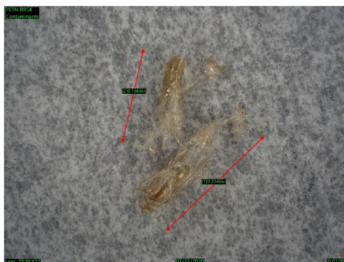
Figure 3. Contaminants removed from the RR5K PETN. Fig. 2 from Ref. 5.
