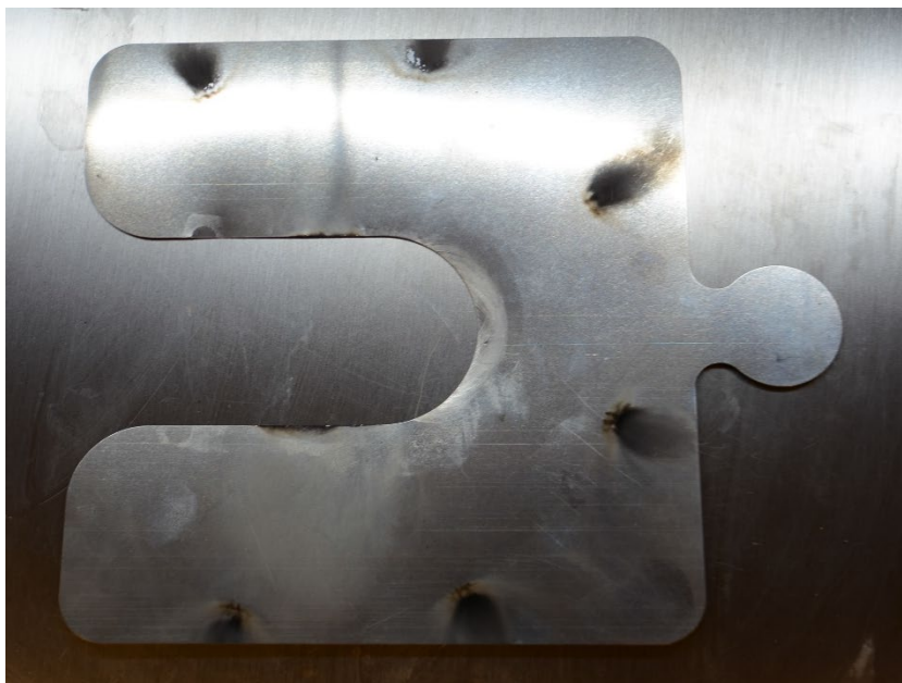
Figure 4. Shim during disassembly showing soot marks corresponding to spanner wrench holes in the Cap.
