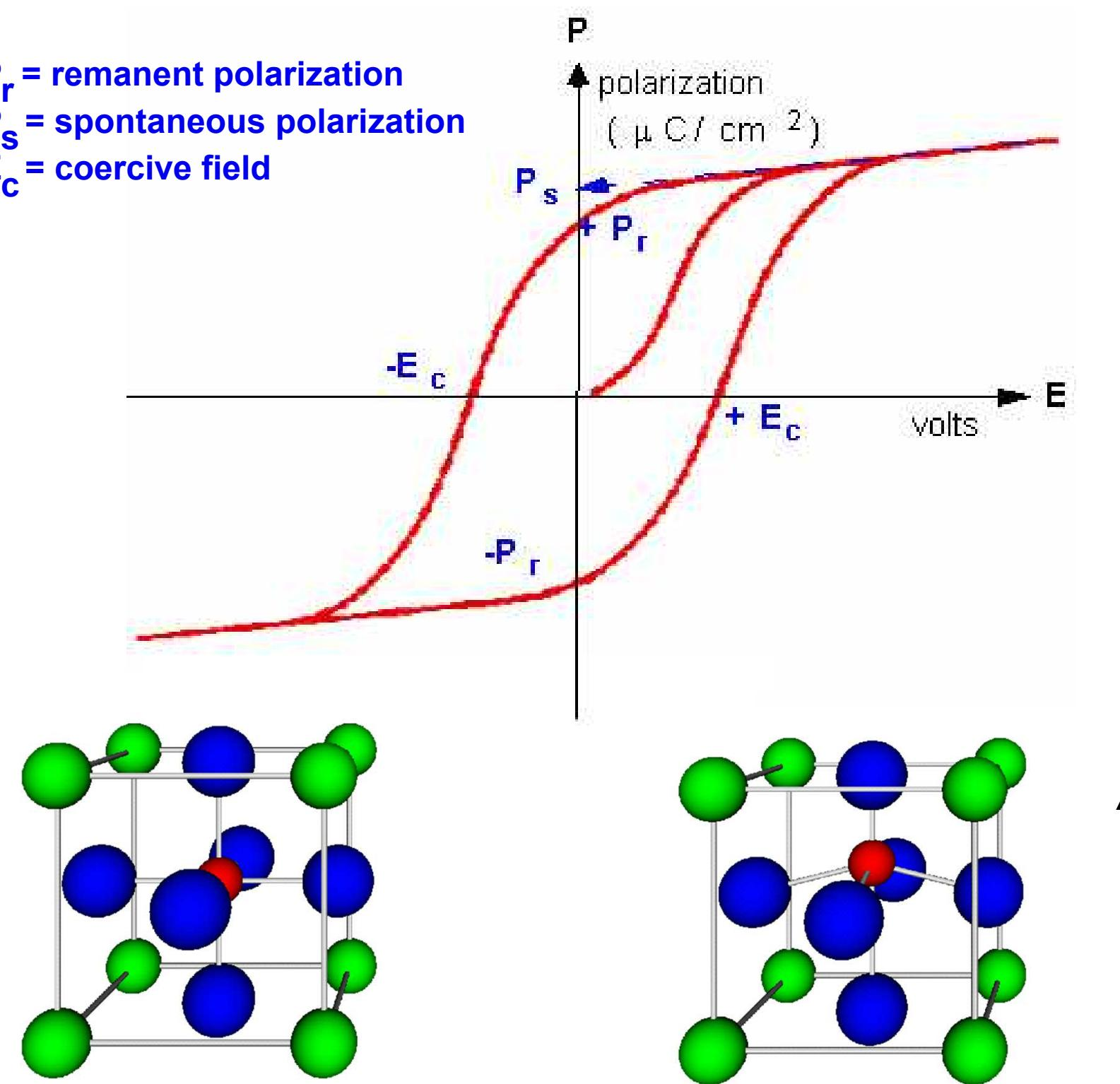
Lead Zirconium Titanate (PZT) is a common ferroelectric used in computer memories. However, PZT tends to fatigue (i.e., wear out) over cycle times greater than  $10^6$  on silica substrates, meaning the B site cation in its perovskite structure stops responding to the electric field as the bond wears out.
