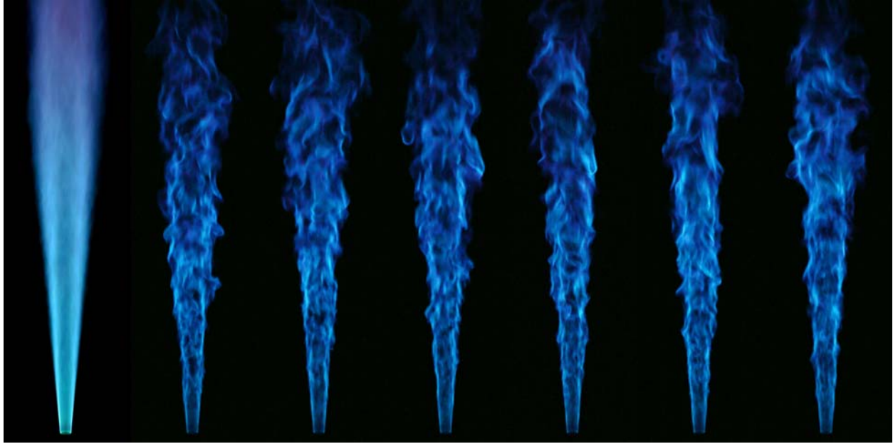
Figure 1. Chemiluminescence images of a turbulent \text{CH}_4/\text{H}_2/\text{N}_2 jet flame ( Re_d = 15,200 ) measured with two different exposure times. The long exposure image (far left) indicates the mean flame structure, and the six shorter exposures to the right illustrate the instantaneous turbulent structure.
