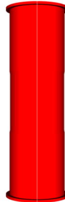
Figure 3.3. Actual and truncated-model pipe geometries. Full length of pipe is 14 inches. Modeled portion omits 1.6 inches from each end of pipe, leaving \frac{1}{4} in. length of stiffening collar at pipe ends. This decreases the finite-element count by almost 30%.
