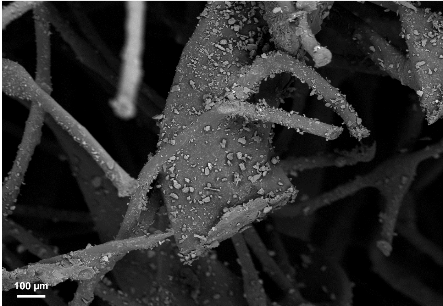
Canister top: heavily loaded with dust
