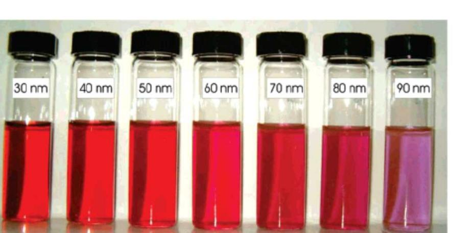
Solutions of gold nanoparticles of difference sizes. Color originates from surface plasmon resonance.
