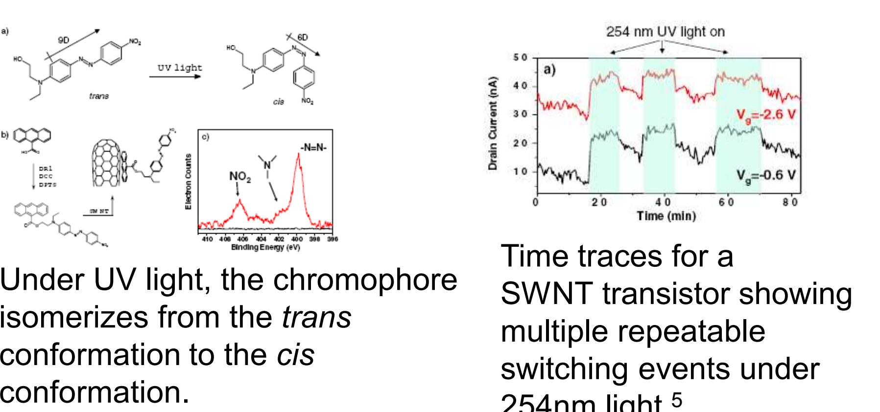
Under UV light, the chromophore isomerizes from the *trans* conformation to the *cis* conformation.
