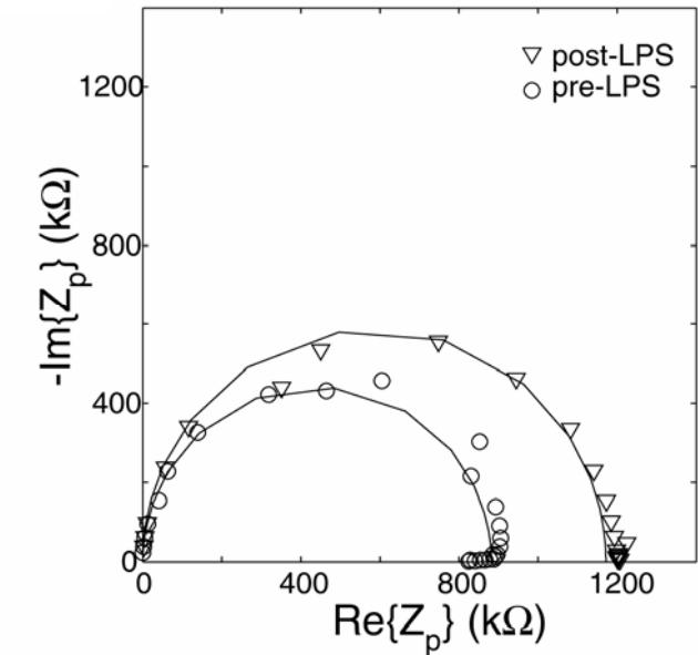
Two mechanisms for an increase in impedance across the microhole: increased spreading (longer path of resistance) and increased adhesion (narrower path of resistance)
