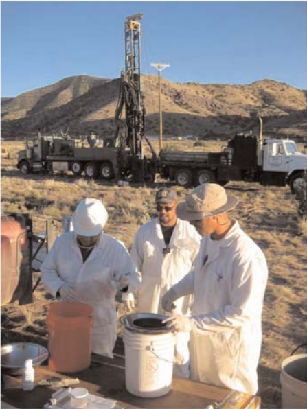
Processing soil collected from Borehole 58FF-GR-BH13 through a brass screen to remove oversized material. Power lines that traverse the Feature 58FF site can be seen behind the drilling rig. View to the southeast, October 23, 2005.
