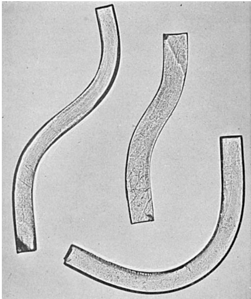
KCl crystals bent by hand
