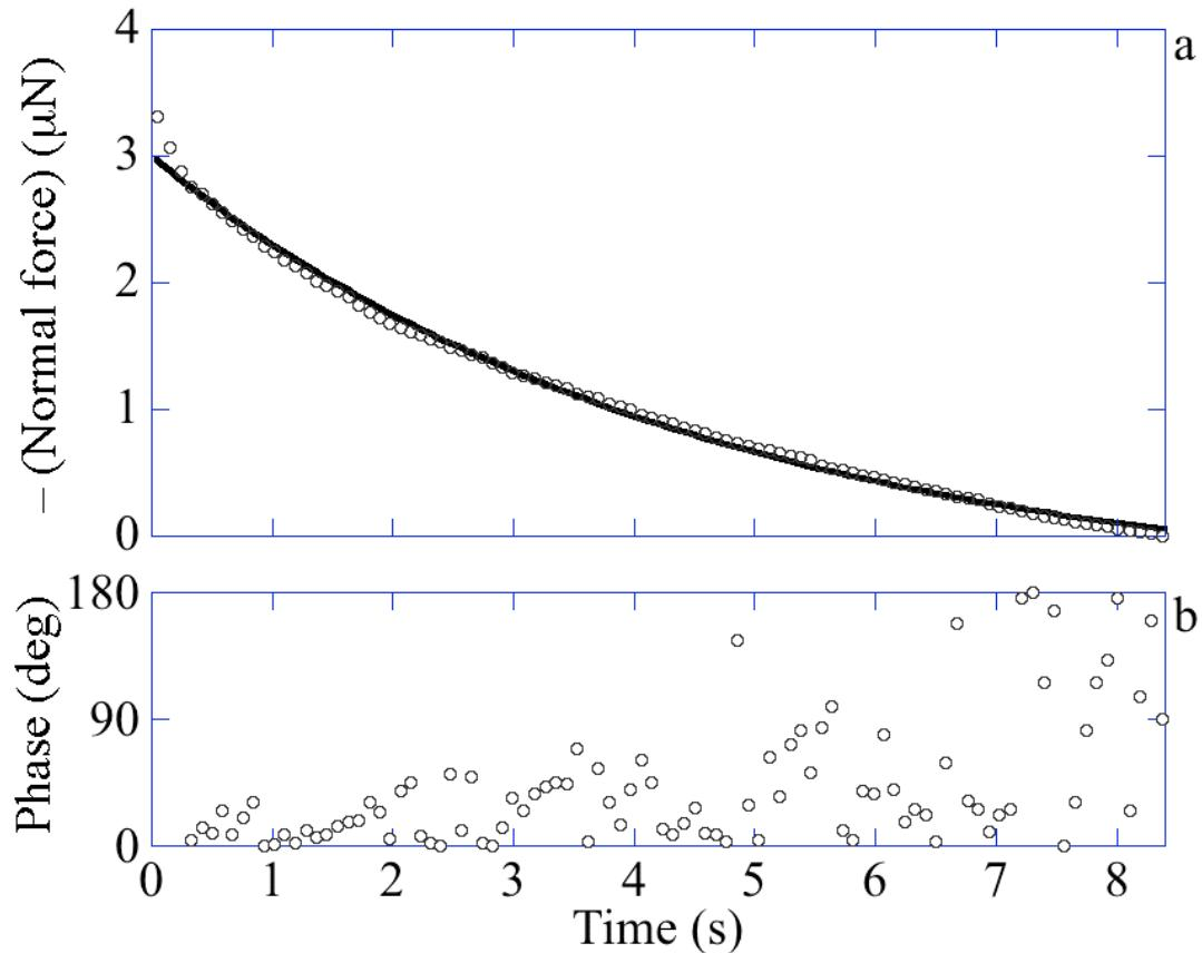
a Nanowire relaxation after imbedding the tip  $\sim 20\text{\AA}$  below the crystal surface and then retracting  $500\text{\AA}$ .
