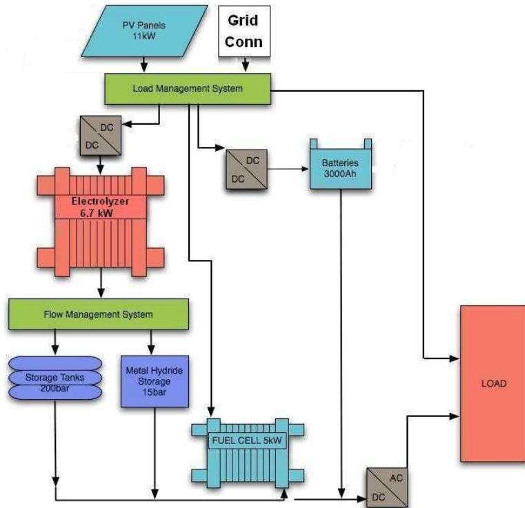
**Figure 1: Technical schematic of the components involved in the hydrogen house**
