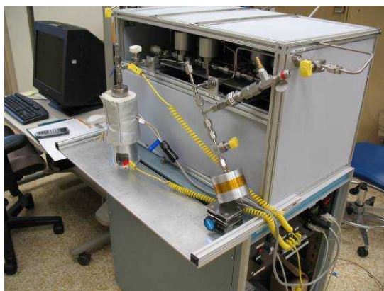
Figure 3 - Automatic Sieverts-style apparatus dedicated to the production of contaminated and un-contaminated samples
