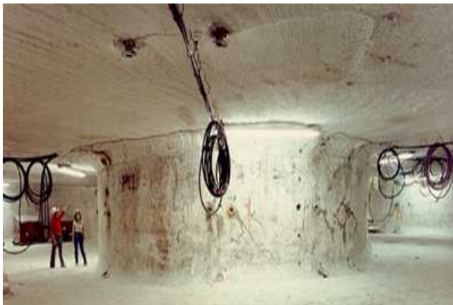
Axisymmetric pillar test
