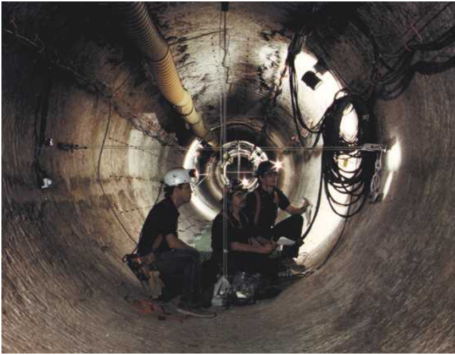
Measurement of creep closure in cylindrical tunnel
