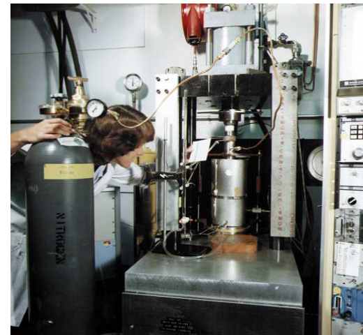
Measurement of creep deformation in the rock mechanics laboratory
