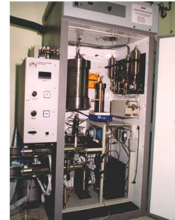
Measurement of 2-phase properties of low permeability rock
