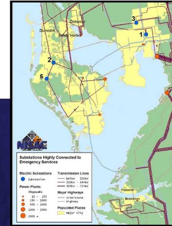
Substations within the 75-100% outage area most highly connected to police stations
