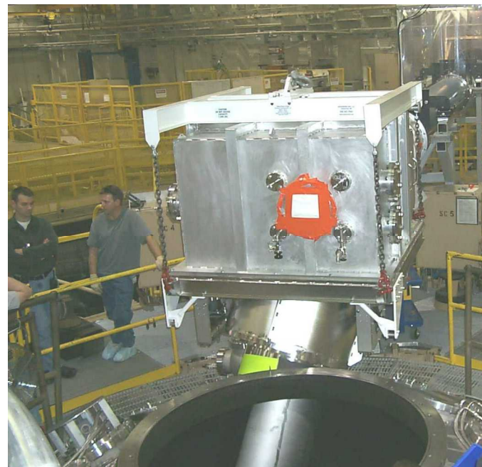
Final Optics Assembly Installed on Z
