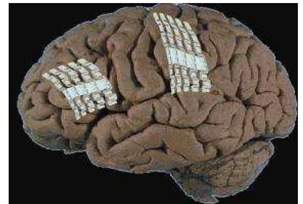
1 mm 24.5:1 Scale Implantable Compliant Electrode array for use in cortical recording and stimulation. (Sandia National Labs)
