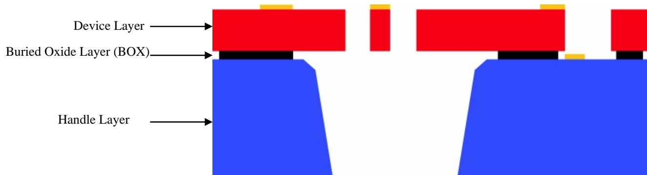
Cross sectional view showing all layers of the SOI-MUMPs™ process (not to scale) SOIMUMPs Design Handbook, Revision 4.0, MEMSCAP
