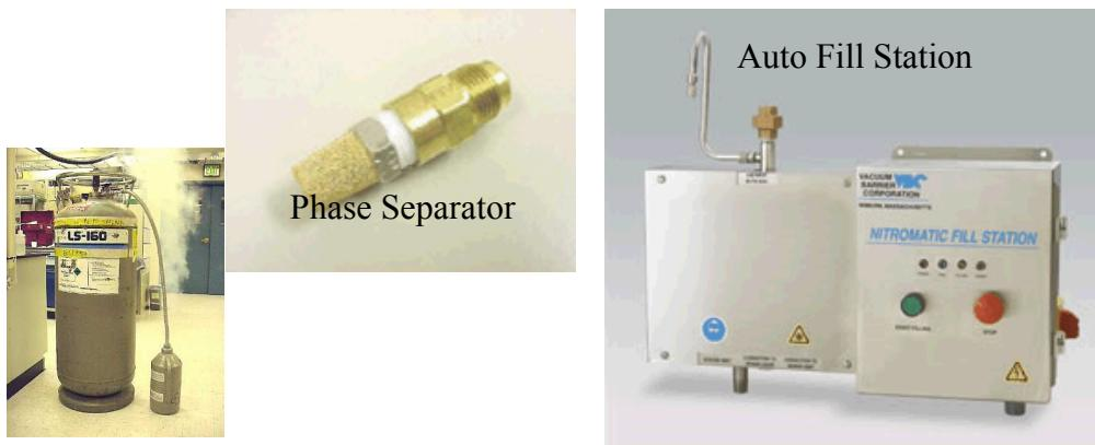
**Do NOT** leave manual valves open and unattended when filling Dewars. Large volume accidental releases have occurred when users left the area – intending to come back in a few minutes. Inevitably, some distraction will cause the user to forget about the open valve, leading to overfilling and the resultant potential hazards of asphyxiation, freezing of floor materials and nearby equipment, etc. This concern is greatest for filling operations inside a building and from a large volume source.
