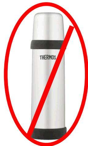
Containers for cryogen applications must be properly rated for the application. Do NOT use consumer containers (such a Thermos bottle) to contain cryogens. Although the Thermos bottle is capable of holding a cryogenic liquid, it would be unsafe to use it in a cryogenic application. The lid design does not allow for proper venting of the boil-off gases and the vacuum space does not incorporate overpressure protection.
