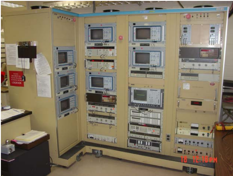
Figure 31. Comparison of PT3697 FE NG Acceptance Tester (old) on left vs. PT3700 FE NG Acceptance Tester (new) on right.
