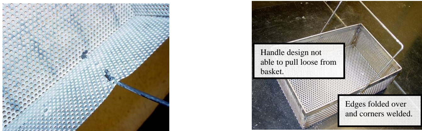
Figure 20. Basket for Holding Encapsulation Parts to be Cleaned Before (left) and After (right) Mistake Proofing
